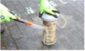
Rinsing the membrane fibre bundles
