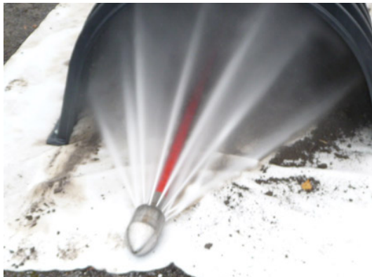
Image 3: Flushing nozzle with reverse conical jets
