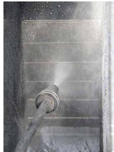
Fig. 20: Cleaning the surface of sieve with high pressure cleaner
