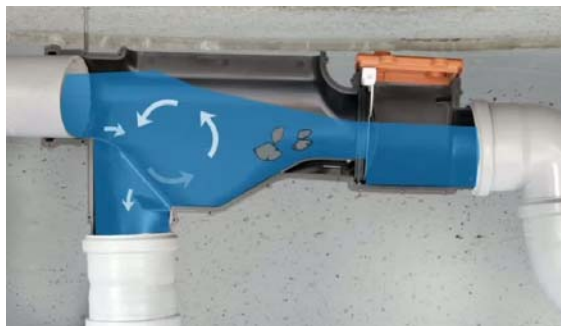
Fig.2: Filtration with hydraulic jump
