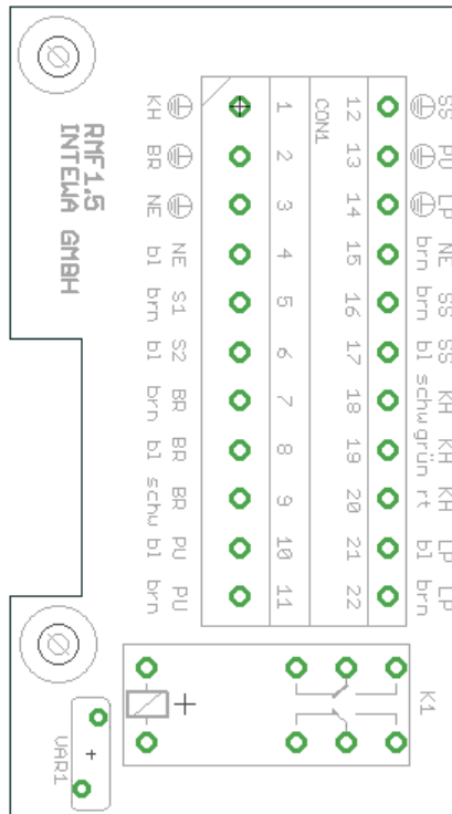
Wiring of the pump terminal
