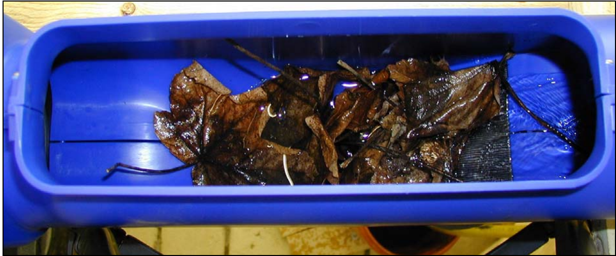
Figure 6: INTEWA Hydraulic jump filter WSP100 with Q = 0.2 l/s with contaminant
