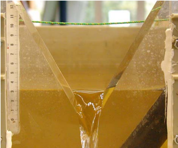
Figure 2: Thompson slope with Q = 0.1 l/s
